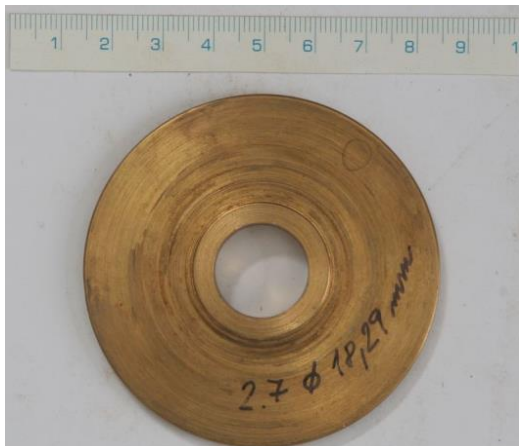
Fig. 5 Example of the orifice with regular opening shape, screen diameter is 18.29 mm.
