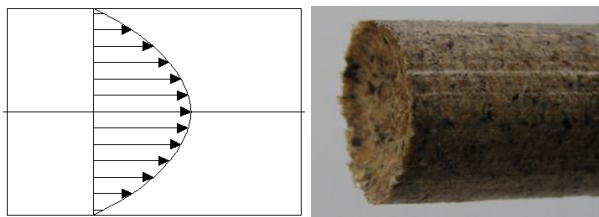
Fig. 8 Pressing force distribution across the pressing chamber
