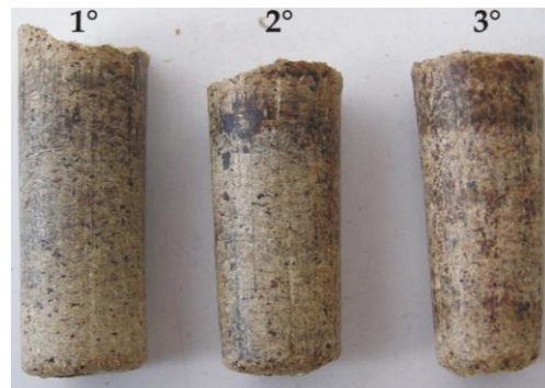
Fig. 7 Negatives of internal chamber space representing different geometries
