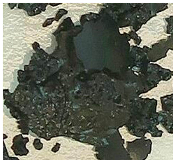
Fig. 6. Asphalt-like solid carbonaceous residue.
