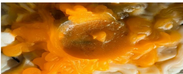
Figure 8 Wax on Low sulphur fuel [74]
