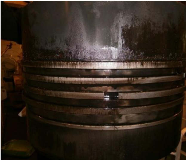
Figure 2 Hard Calcium deposit on piston [46]
