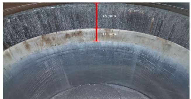
Figure 7 Photograph of the surface of a used cylinder liner. The upper 18 mm is covered by a protective “coked” lube oil layer. Wear can be seen in the swept liner surface 11 mm below the top. Post that surface where honing is done can be seen [64]
