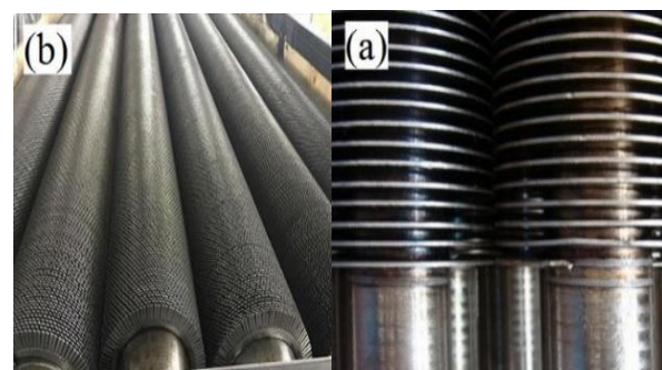
Fig. 3 Type of finned tubes HFRW process (a) Solid finned tubes (b) Serrated finned tubes
