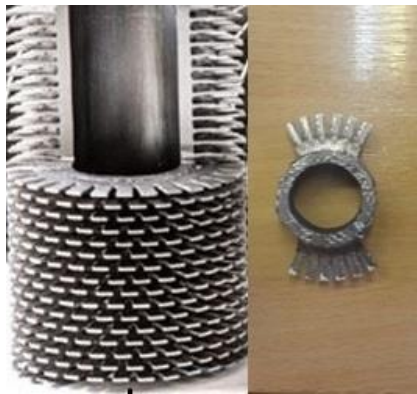
Fig. 4 Sample tests preparation of 2¼ Cr-1 Mo seamless tube and A240TP409 finned tubes
