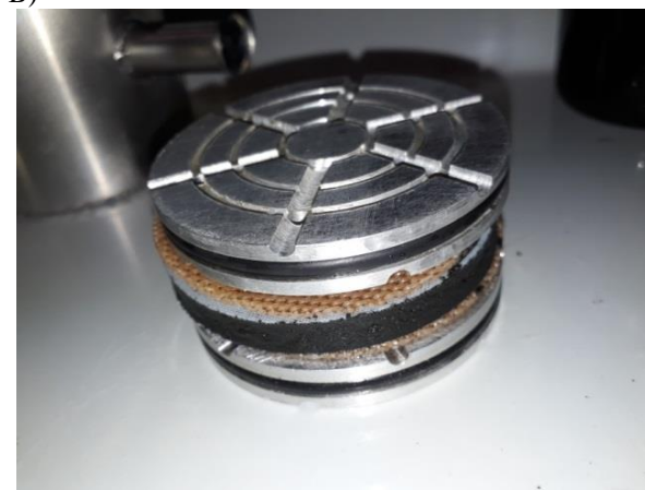
Fig 1 A- the machine Mareco minipress MMP-3/2 used during filter pressing method; B – sludge cake after pressing.
