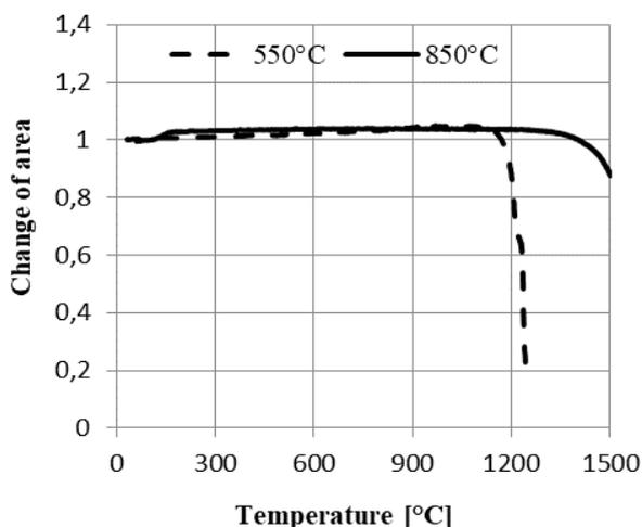
**Figure 4.** Observed difference in ash melting tendency
