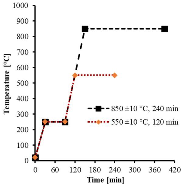
**Figure 2.** Ashing and conditioning of *Acacia Mangium* test portions in the different empirical conditions
