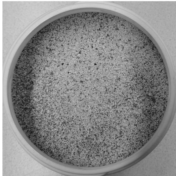
**Figure 5** Mixture of calcite as bed material
