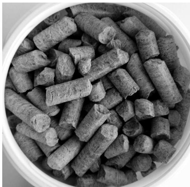
**Figure 6** Typical feedstock pellets size 6-8mm
