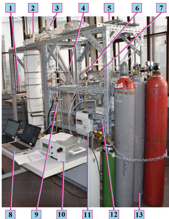
Fig. 2 Front right view of the apparatus A (1 – furnace controller, 2 – reactor, 3 – recuperation heat exchanger/candle filter, 4 – water plate cooler, 5 – air cooler, 6 – manometer, 7 – overpressure compensator, 8 – data collecting laptops, 9 – water flow restrictor, 10 – IR spectrometer, 11 – A/D converter, 12 – membrane gas meter with pulse encoder, 13 – pressure cylinders with gas mixtures)
