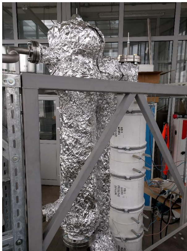
Obr. 3 Fotografie aparatury s fluidní vrstvou sorbentu Fig. 3 Photo of apparatus with fluidized bed of adsorbent
