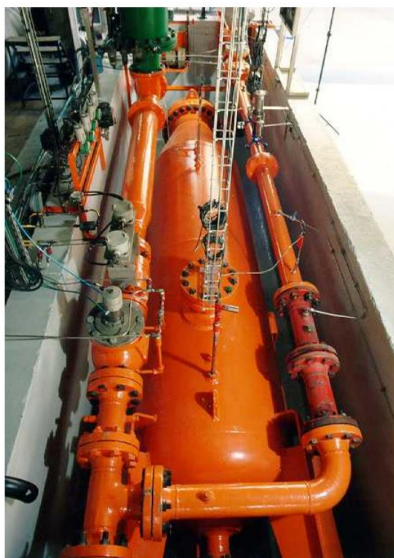
Obr. 8 pVTt standard pro kalibraci Venturiho dýz v LNE LADG [19] Fig. 8 pVTt standard for Venturi sonic nozzles calibration at LNE LADG [19]
