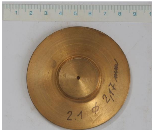
Fig. 4 Example of the orifice with regular opening shape, screen diameter is 2.17 mm.
