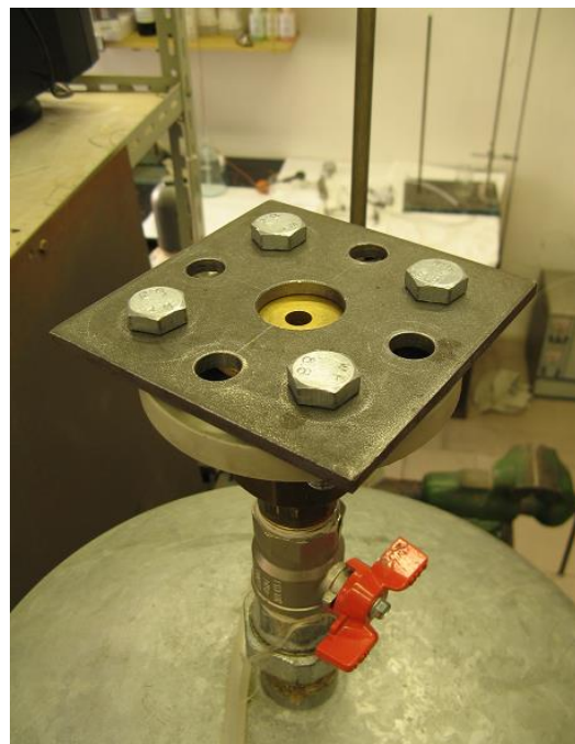
Fig. 3 detail of the flange with a measured orifice
