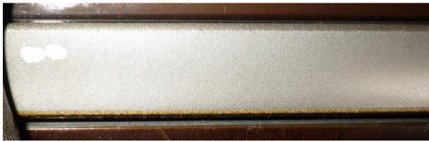
Figure 3 Good condition cermet-coated piston ring
