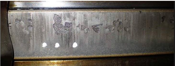
Figure 6 Partly damaged piston ring after hard contact
