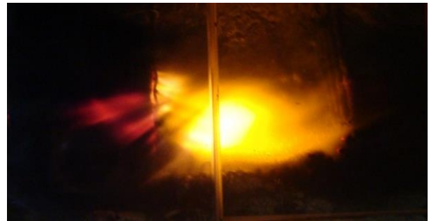
Fig 3 Combustion torch of two-component granules based on sludge and peat: dilution 250 Pa
