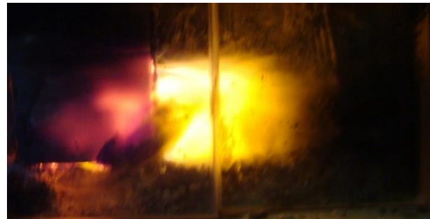
Fig 4 Combustion torch of three-component granules based on sludge, peat and buckwheat husks: dilution 250 Pa
