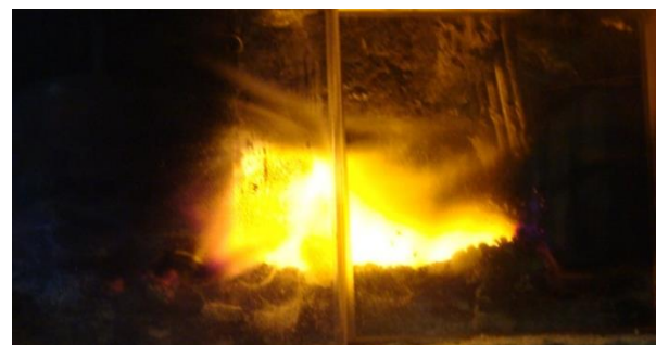
Fig 5 Combustion torch of three-component granules based on sludge, peat and sawdust: dilution 500 Pa
