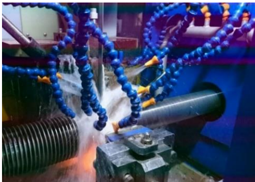
Fig. 2 Manufacturing process of finned tube by HFRW technology
