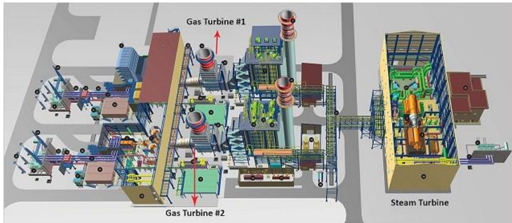
Fig. 1 A block of modern combined cycle power plant (CCPP)
