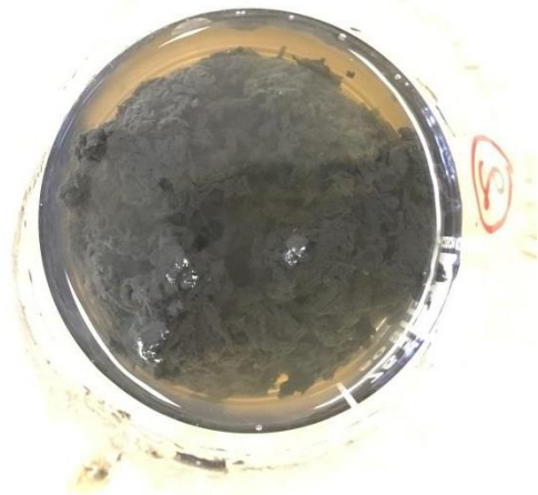
Fig 4 Illustration of non-optimal flocculation process.
