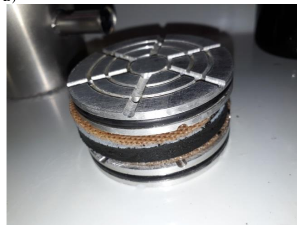
Fig 1 A- the machine Mareco minipress MMP-3/2 used during filter pressing method; B – sludge cake after pressing.
