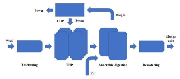
Fig 1 Integration of thermal hydrolysis process in sludge processing technology. Thermal hydrolysis of only waste activated sludge (WAS), while primary sludge (PS) is thickened and further added to hydrolyzed WAS before entering anaerobic digestion.
