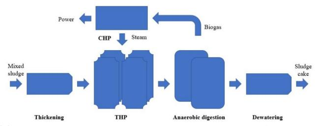
Fig 2 Integration of thermal hydrolysis process in sludge processing technology. Thermal hydrolysis of mixed sludge.
