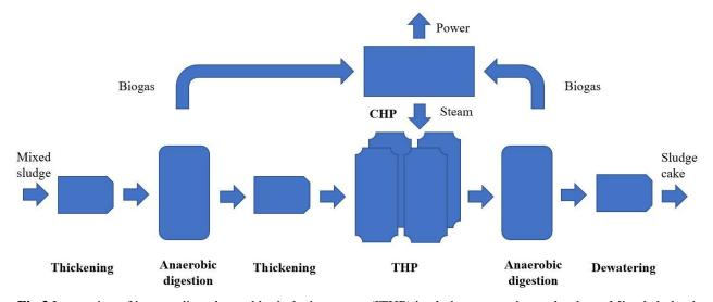
**Fig 3** Integration of intermediate thermal hydrolysis process (ITHP) in sludge processing technology. Mixed sludge is first stabilized in the first anaerobic digester, then hydrolyzed in ITHP and then digested again in the second digester.
