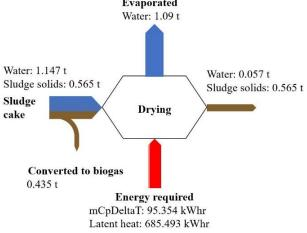
**Fig 7** Sankey diagram of hydrolyzed sludge – energy balance – overtaken from [4]
