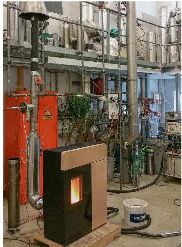
Figure 1. Test bench assembly with horizontal flue outlet
