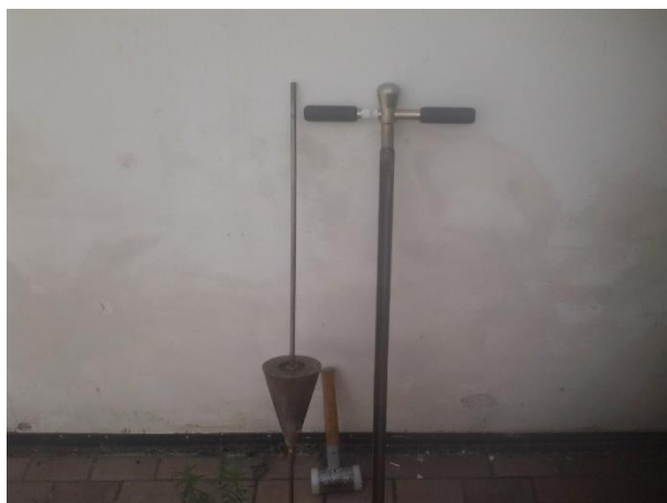
Figure 2: Sampling set for atmogeochemical survey
