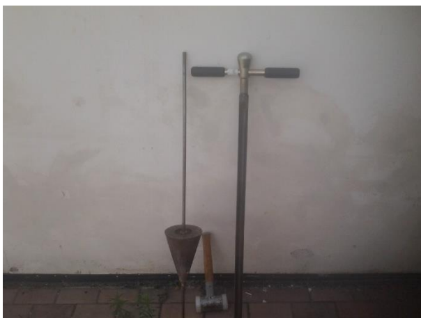
Figure 2: Sampling set for atmogeochemical survey
