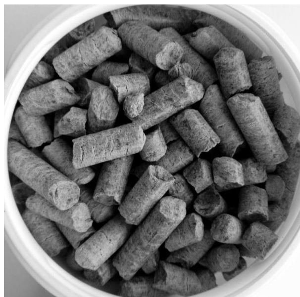
Figure 6 Typical feedstock pellets size 6-8mm
