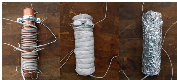
Figure 2 Fabrication of a furnace
